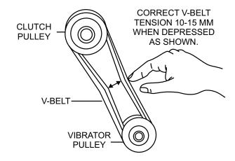
Figure 8. V-Belt Tension
